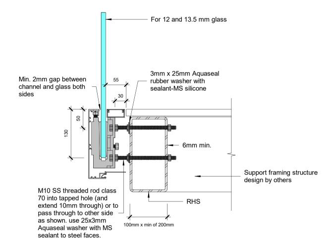
Steel members to be designed by Engineer CPEng. Spacing limited by glass capacity - refer to PS1 certificates
